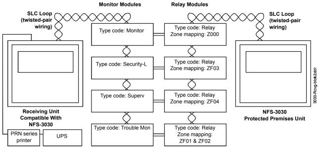
Note: Remote printers require 120 VAC, 50/60Hz primary power. A secondary power source (battery backup) is not provided; the use of a separate Uninterruptable Power Supply (UPS) 50 watt minimum, UL-listed for Fire Protective Signaling is recommended. A UPS is required for NFPA 72-1999 Proprietary Protected Premises Receiving Unit Applications.
