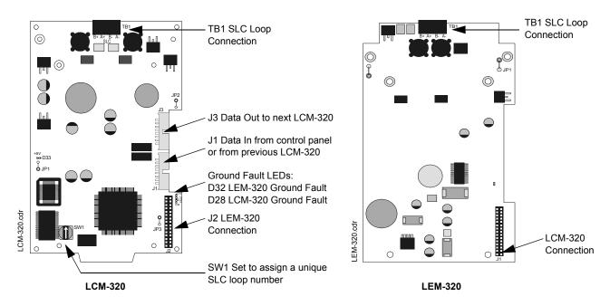
Note: Do not cut any jumpers on LCM-320 or LEM-320
