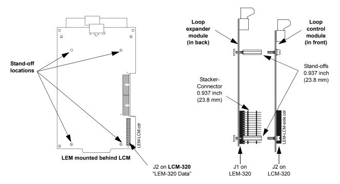
Figure 25 Inserting LCM-320/LEM-320 into CHS-4L
