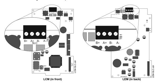
Figure 27 Connecting Multiple LCM-320/LEM-320 Pairs
