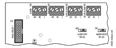
SW1 set to Security SW2 set to Supervisory Move switch to opposite position to convert to Alarm relays.
