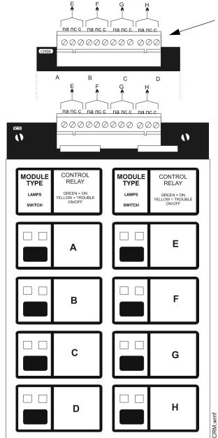
\* Optional CRE-4 Control Relay Expander. Positions E, F, G and H are active only with this board installed.
