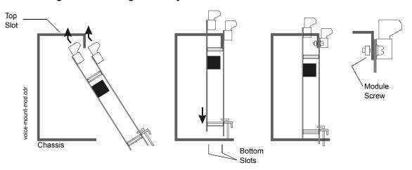
**Note:** Depending on system components, clearance may be tight. Do not force modules! Move the assembly around gently until you find the angle where components and mounting studs pass each other without scraping together.
