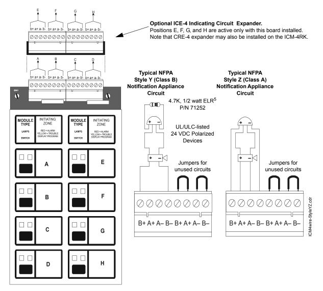
Figure 15 Field-Wiring an ICM-4RK/ICE-4: NFPA Style Y, Z
