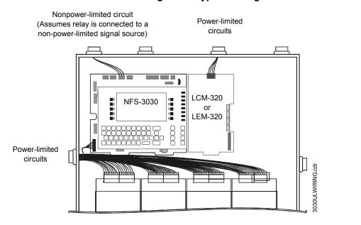
Figure 29 Typical Wiring in a Four-Row Backbox
