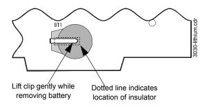
This battery's shelf-life should exceed 10 years, but if for some reason it fails, the control panel will show a trouble when powered up. To replace the lithium battery:
