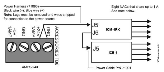
**Note:** For limitations on the total current available for any group of Notification Appliance Circuits (NACs), see Section 3.13 "Notification Appliance Circuit Current Limitations" on Page 35, as well as the manual for your system's power supply.
