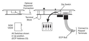
Figure 3-21: Wiring the FSA Module
