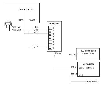
Figure 3-26: Wiring the 4100APG With the Serial Printer
