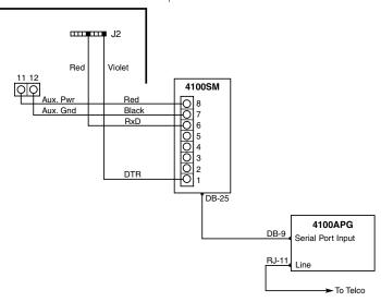
Figure 3-25: Wiring the 4100APG Without the Serial Printer
