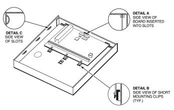
Figure 3-3: Mounting the PC Board
