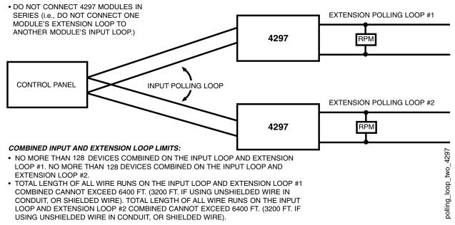
Figure 3-16: Polling Loop Connections Using Multiple Extender Modules
