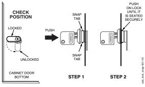
Figure 3-1: Installing the Lock
