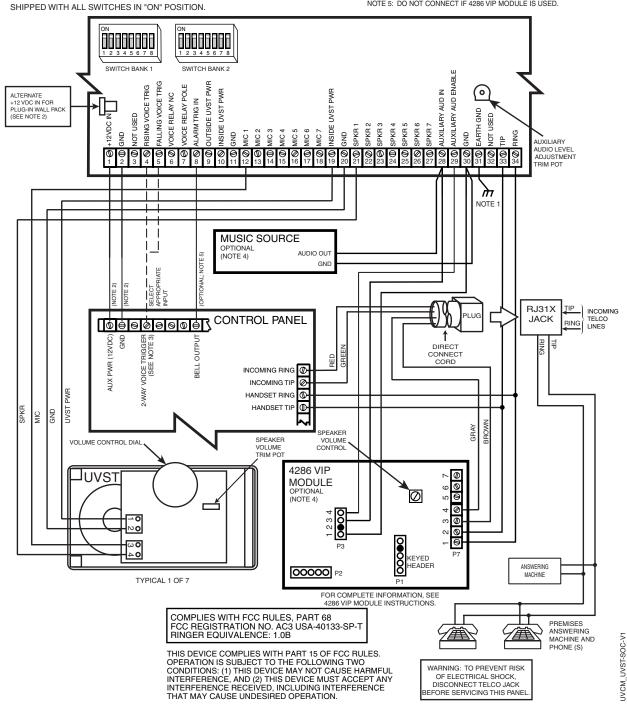
Figure 3-31: UVS Connections to the Control Panel
