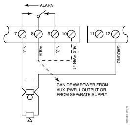
Figure 3-7: Wiring Auxiliary Relay for Alarm Activation
