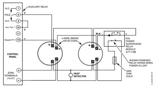
Figure 3-8: Wiring Auxiliary Relay for Smoke Detector Reset
