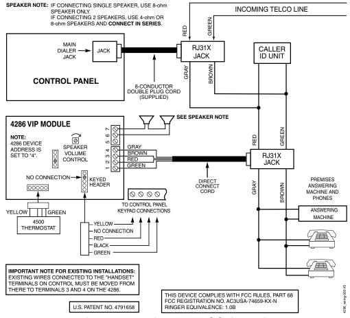
Figure 3-30: 4285/4286 VIP Module Connections
