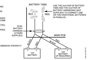
Figure 3-32: Connecting the Backup Batteries
