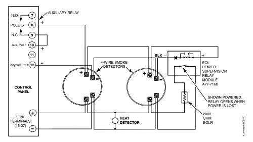
Figure 3-10: 4-Wire Smoke Detectors
