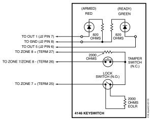
Figure 3-22: Remote Keyswitch Wiring
