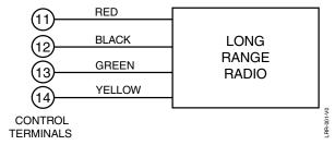
Figure 3-24: Wiring Long Range Radio to Keypad
