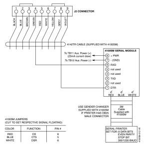
Figure 3-29: Printer Connections to the 4100SM
