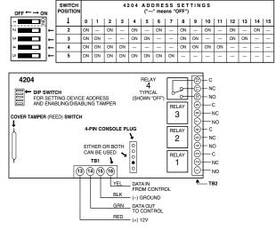
Figure 3-19: 4204 Relay Module
