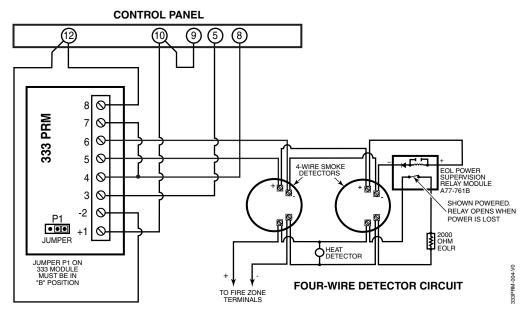
Figure 3-11: Wiring a 333PRM to the Control
