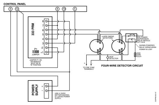
Figure 3-12: Wiring a 333PRM using a Power Supply
