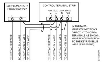
Figure 3-5: Using A Supplementary Power Supply
