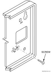
Figure 3-17: Installing the 5881ENHC with Tamper Protection
