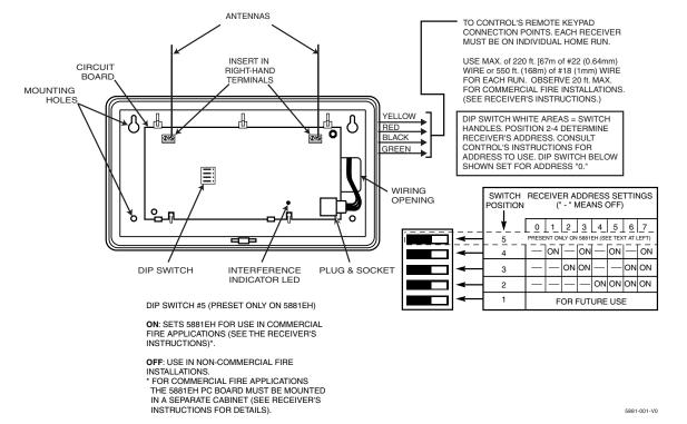
Figure 3-18: 5881 RF Receiver (cover removed)
