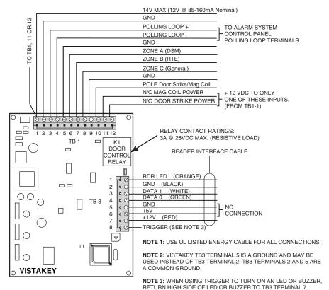
Figure 3-27: Wiring the VistaKey
