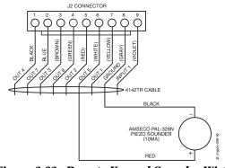
Figure 3-23: Remote Keypad Sounder Wiring
