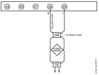
Figure 3-14: Polling Loop Connections to the Control Panel
